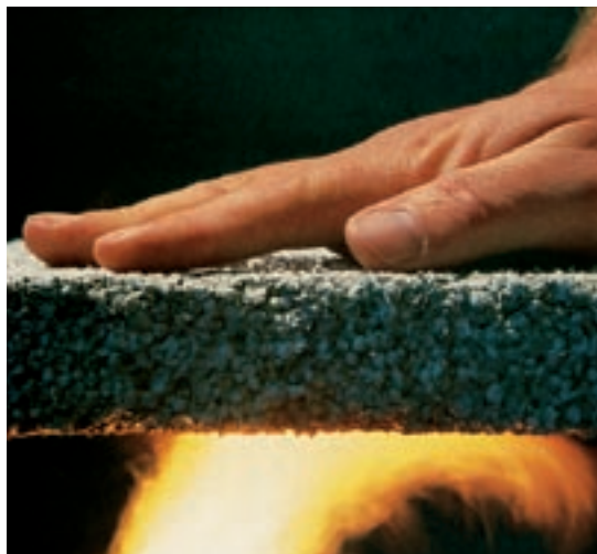
Concrete provides protection against heat from fire.
